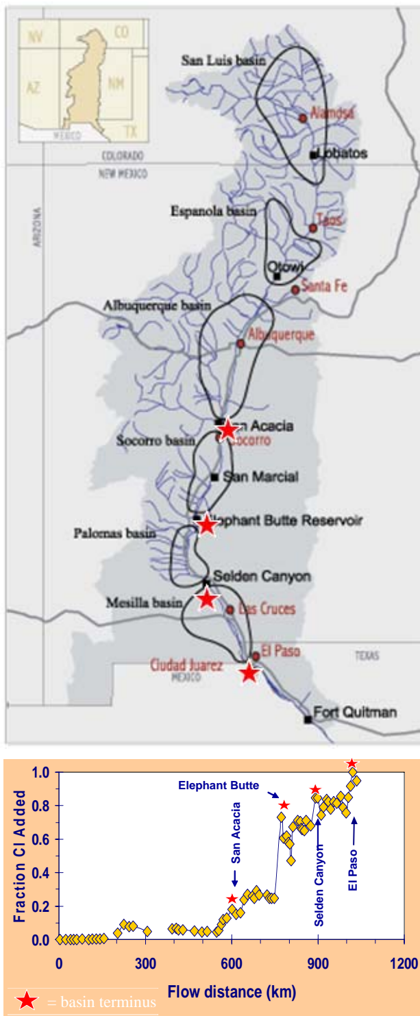
Figure 5. Points of salt addition; rraction Cl added vs flow distance
